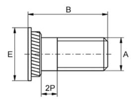
For plate thickness, min = 1.5Head diameter E = 6Hole diameter +0.1 = 4.2
